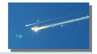
Columbia explodes during re-entry due to damage done to left wing caused by broken foam.
